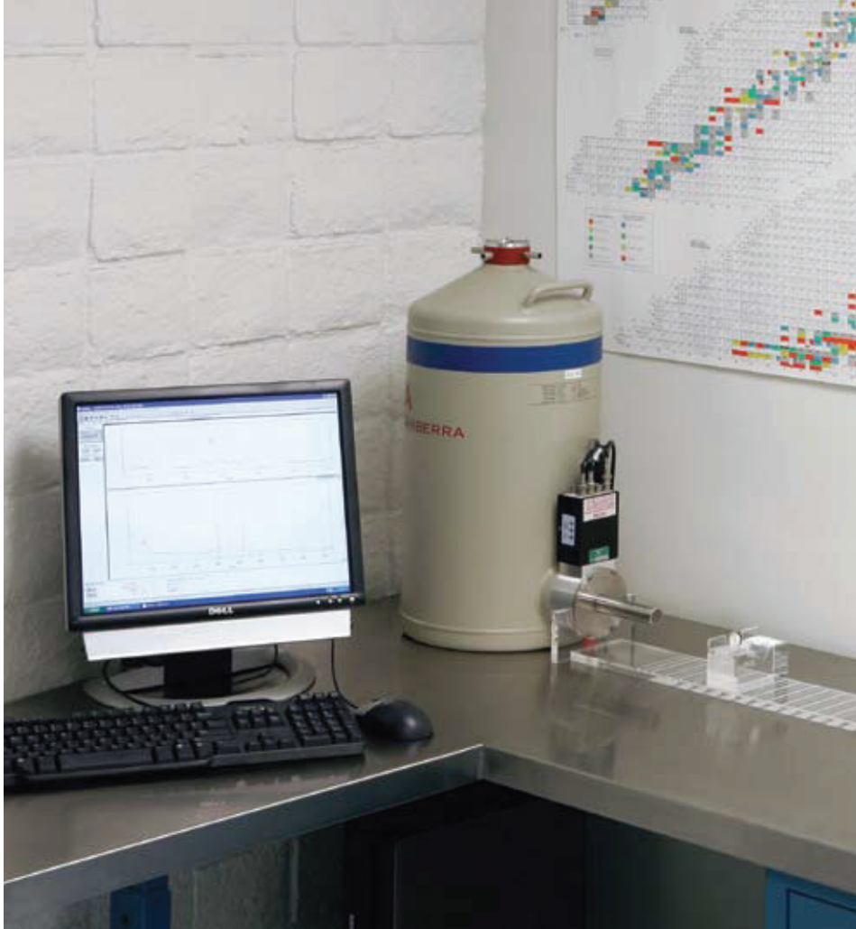
Eckert & Ziegler Isotope Products precisely measures the output of each source prior to dispatch.
